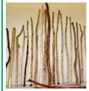
Good, safe woodworking takes time. Begin by trimming off twigs with a garden pruner or handsaw. Keep the bark on the stick if you wish or whittle off the bark to make a bare wood stick. First, smooth off any bumps or rough spots by shaving with a pocketknife, or a plane, or using a fine rasp or coarse sandpaper. Use short, shallow strokes to avoid digging into the wood. Make the stick smooth to the touch with fine sandpaper.
